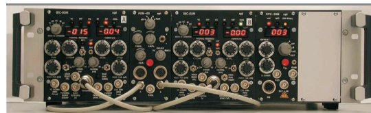
EPMS 07H modular system with seven slots SEC-03M channel A sharp ME, whole cell or perforated patch recordings PENETRATION module for channel A, B, or high-voltage module SEC-03M channel B sharp ME, whole cell or perforated patch recordings High voltage module for two electrode clamp or ultra-fast iontophoresis Spare slot Filter, or stimulus isolator, or CellWorks interface
